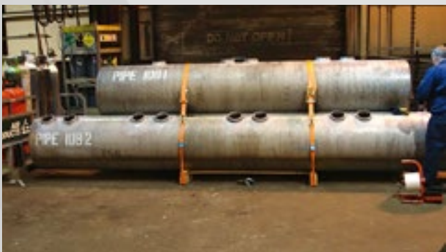
Extruded Manifolds Material : Alloy 800 HT Client : Total Petrochemicals Gonfreville
