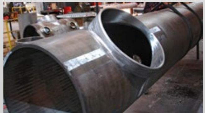
Extruded Manifolds Material : Alloy 800 HT Client : Total Petrochemicals Gonfreville
