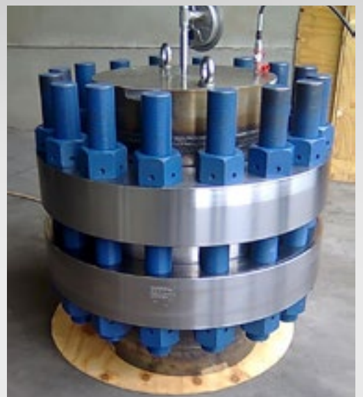
Hydrotest on CF assembly Block 17 phase 2 Total Angola
