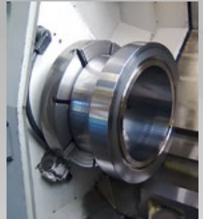
Inhouse machining swivel hubs Tailor made design based on Norsok L-005
